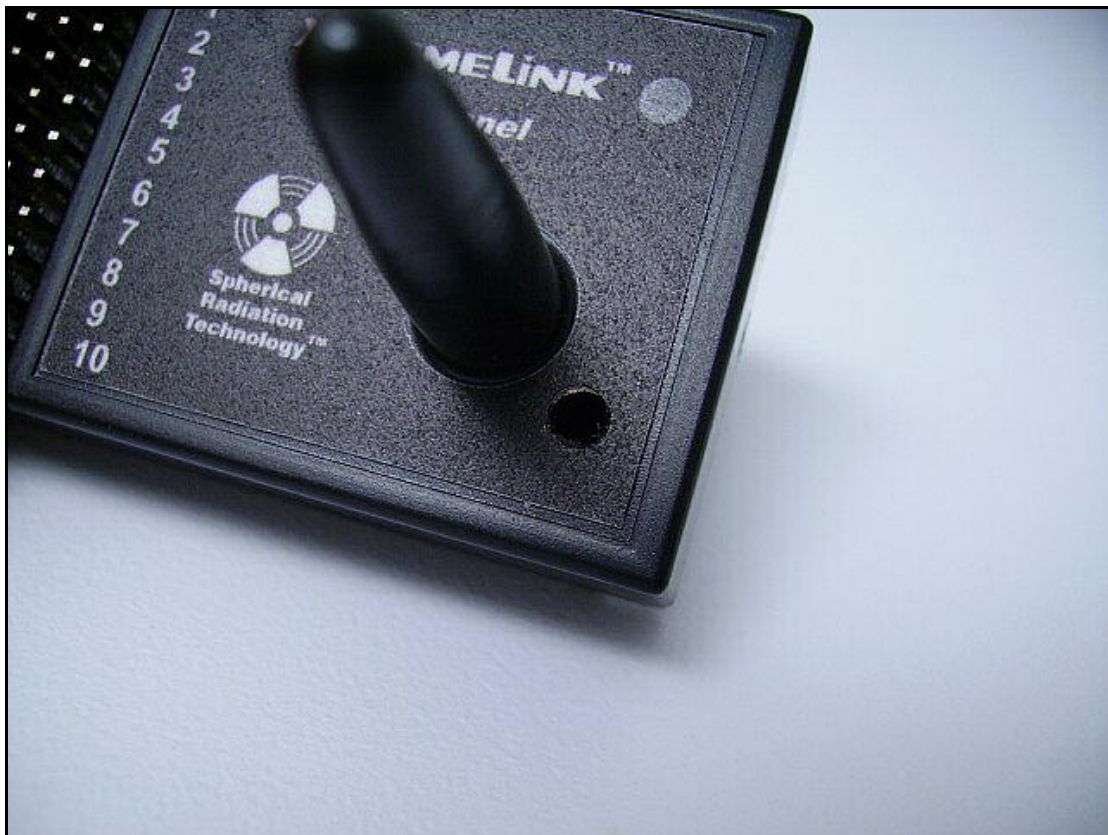
Figure 1 – XtremeLink™ receiver programming button location
