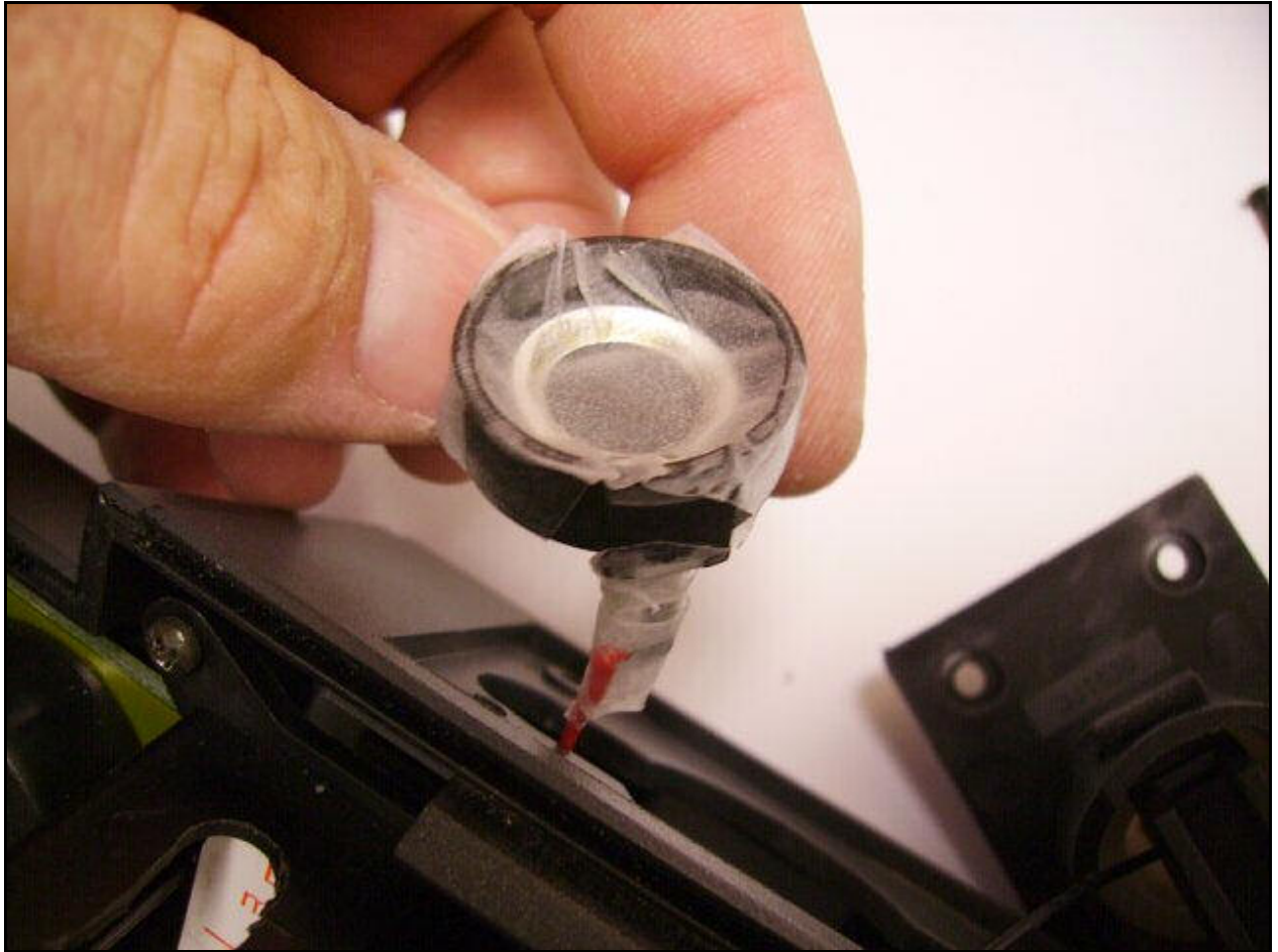
Figure 10 – Antenna base taped
