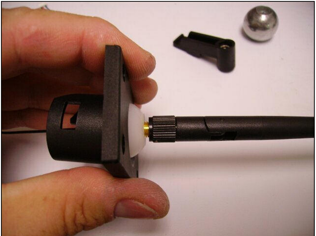
Figure 8 – Ball pulled through using antenna
