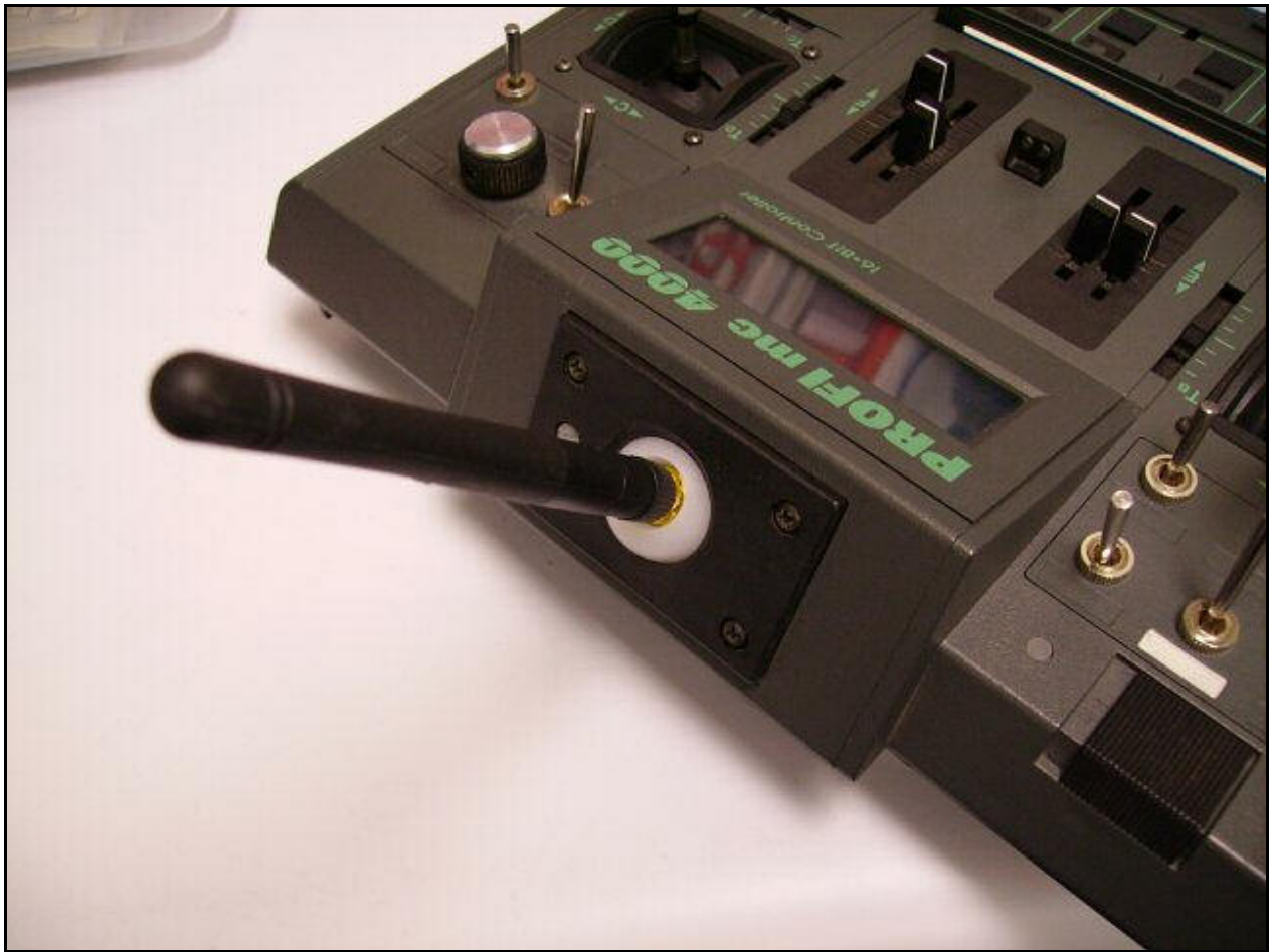
Figure 12 – Completed antenna block
