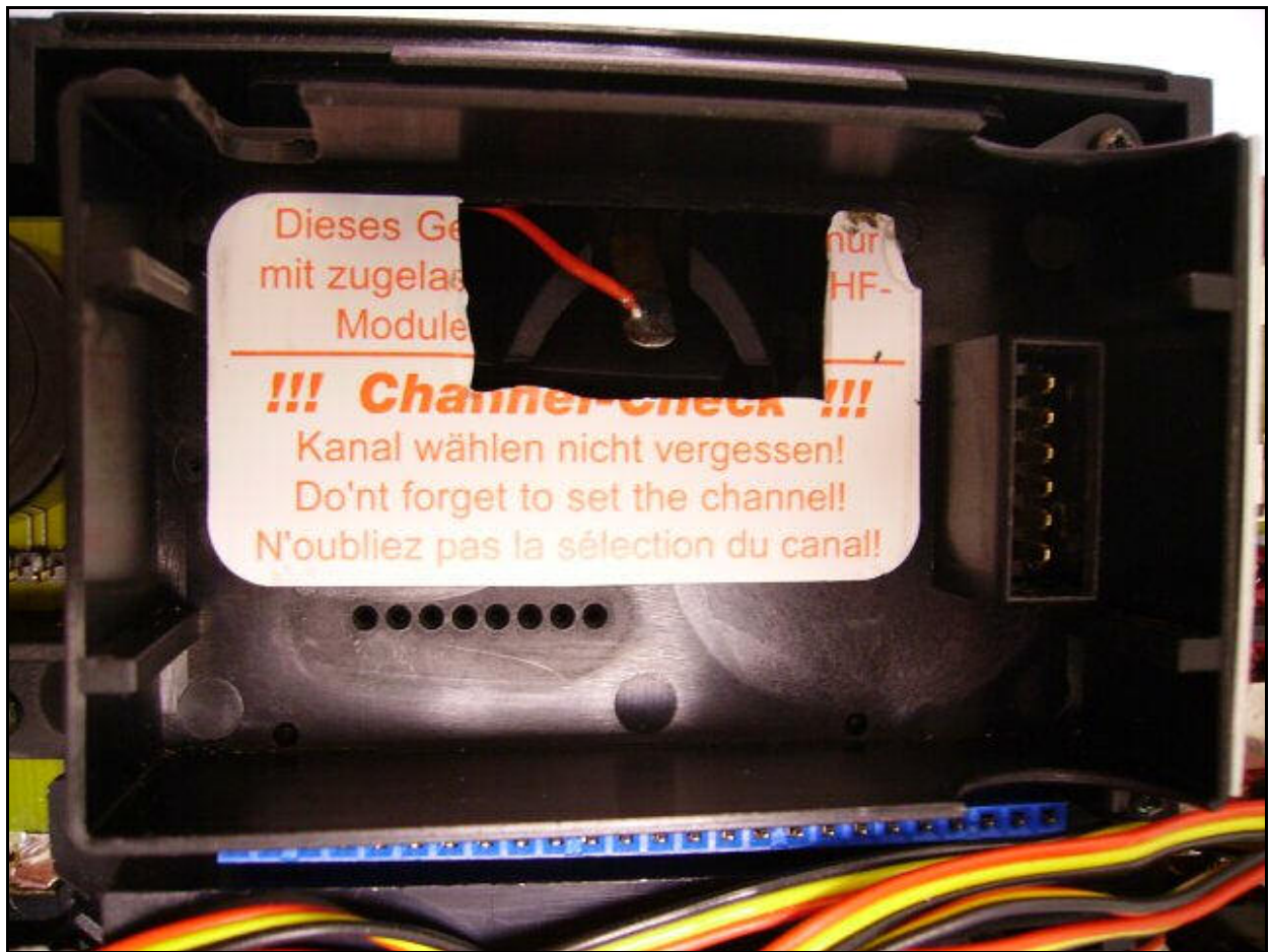
Figure 2 – Warning label cut away to expose antenna access
