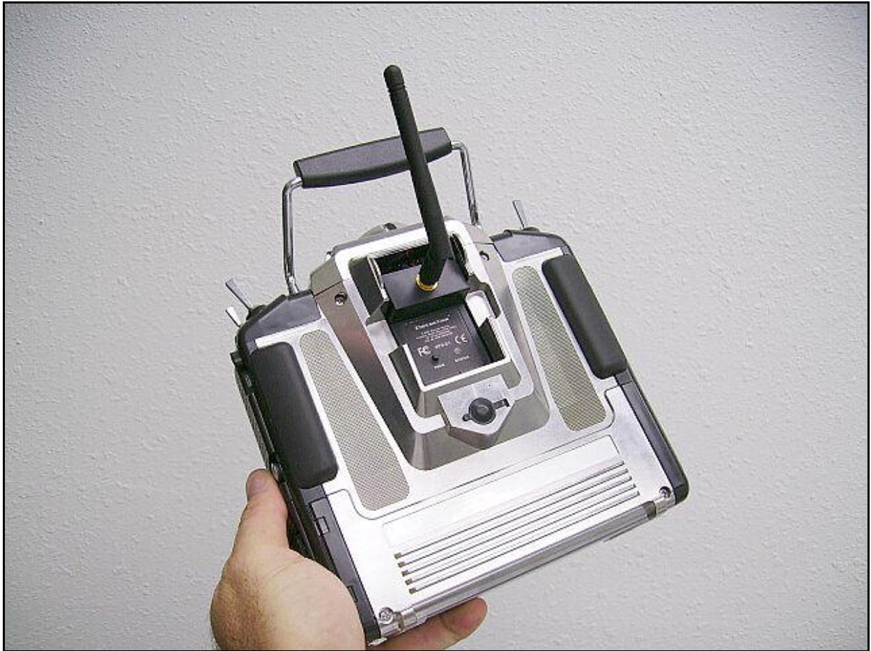
Figure 9 – XtremeLink™ RF module with antenna installed.
