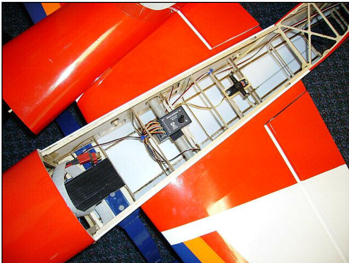
Figure 11 – XtremeLink™ 8 channel receiver installation
