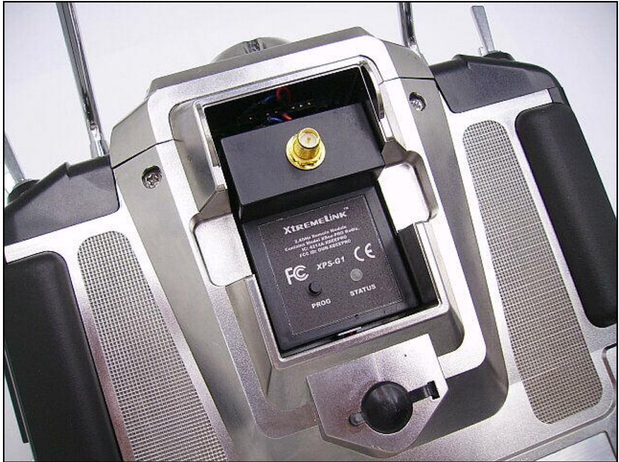
Figure 8 – XtremeLink™ RF module fully installed.
