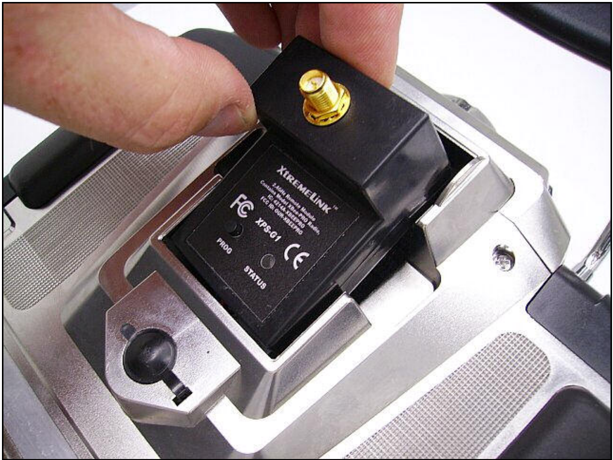
Figure 6 – Insert the bottom of XtremeLink™ RF module first.
