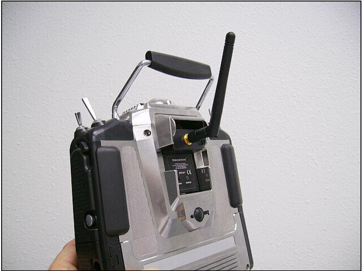
Figure 10 – XtremeLink™ RF module installed.
