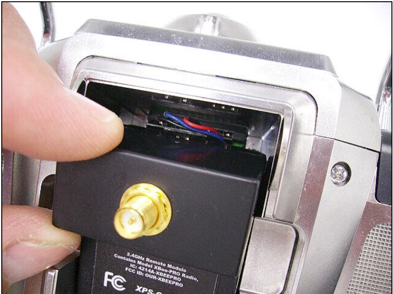
Figure 7 – Carefully push the top of the XtremeLink™ RF module into place.
