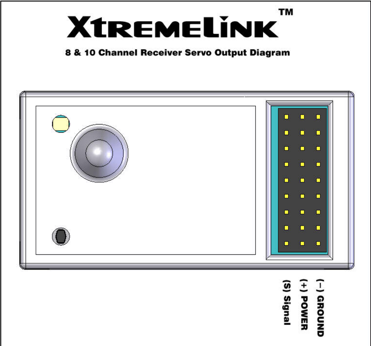
Figure 14 – XtremeLink™ receiver servo output polarity
