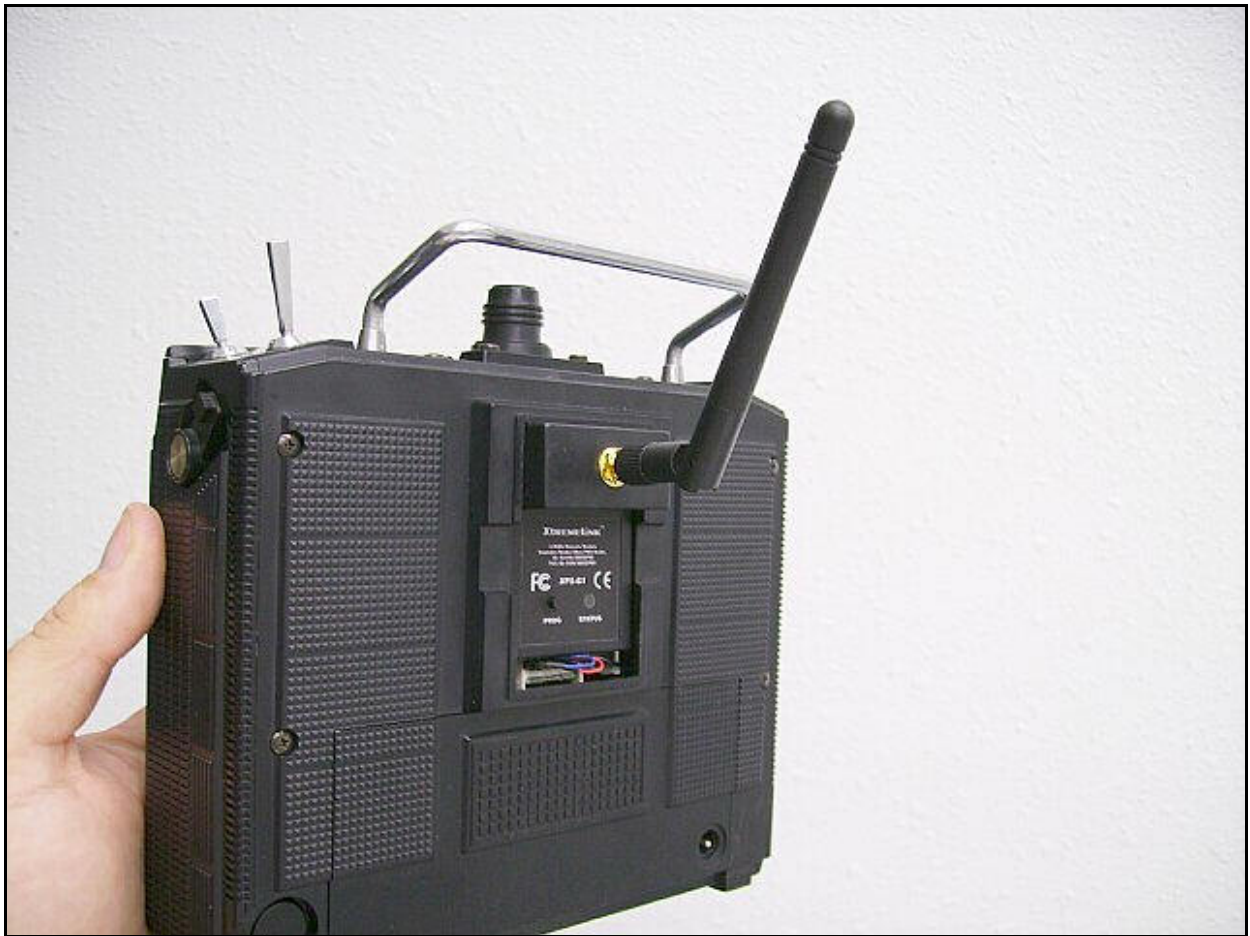
Figure 8 – XtremeLink™ RF module with antenna installed.
