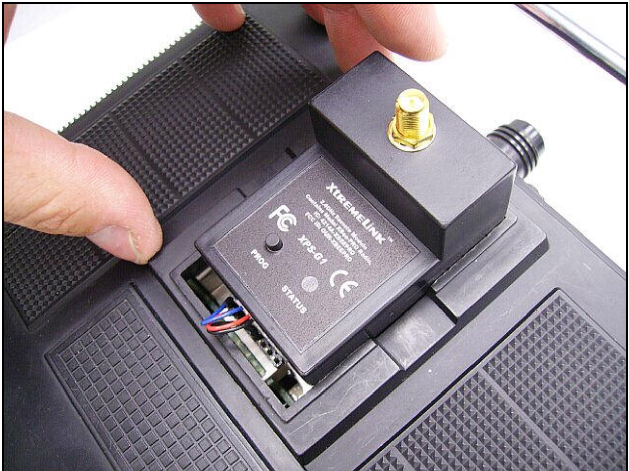
Figure 6 – Carefully push the bottom of the XtremeLink™ RF module into place.
