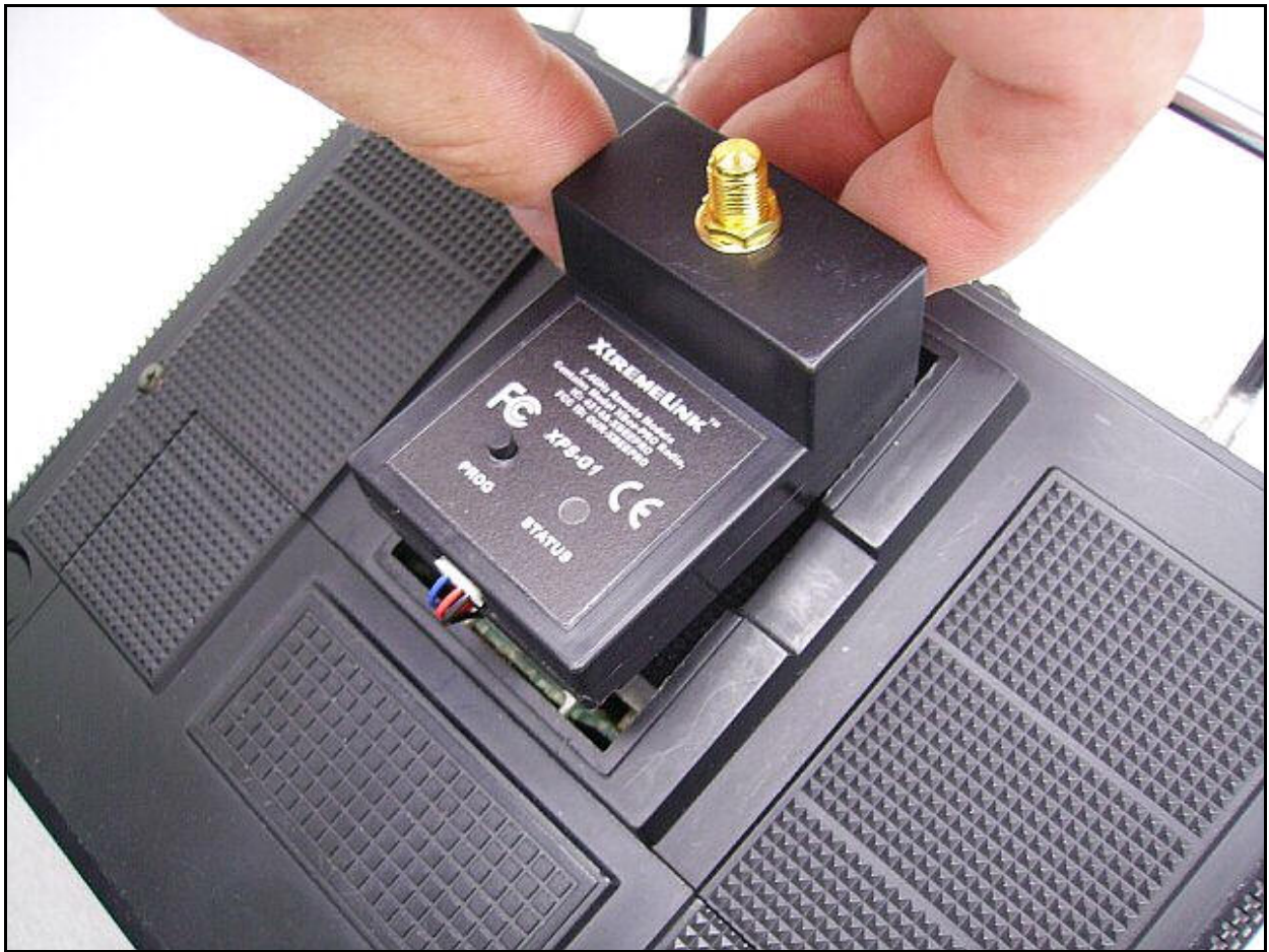
Figure 5 – Insert the top of XtremeLink™ RF module first.
