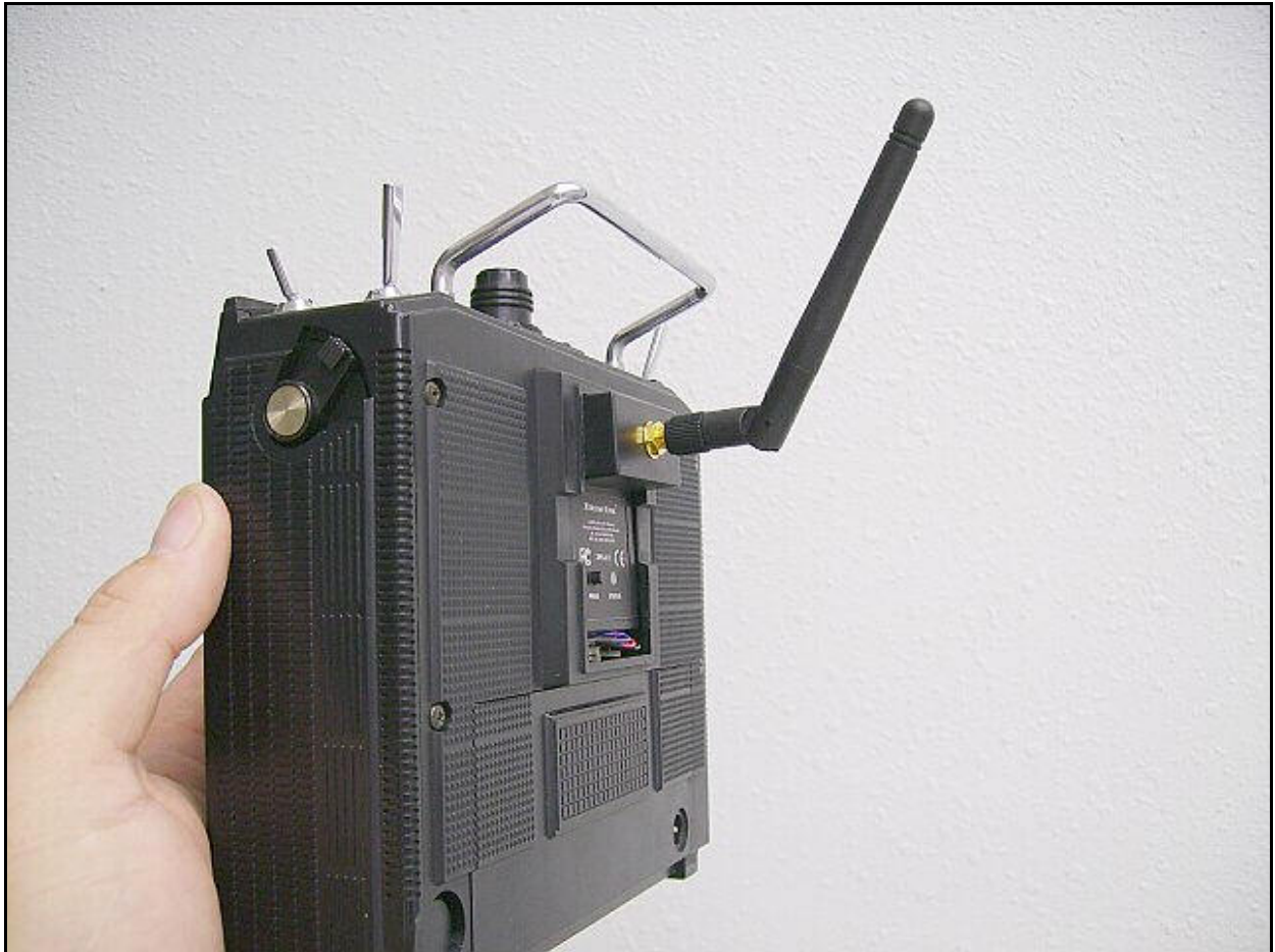
Figure 9 – XtremeLink™ RF module installed.
