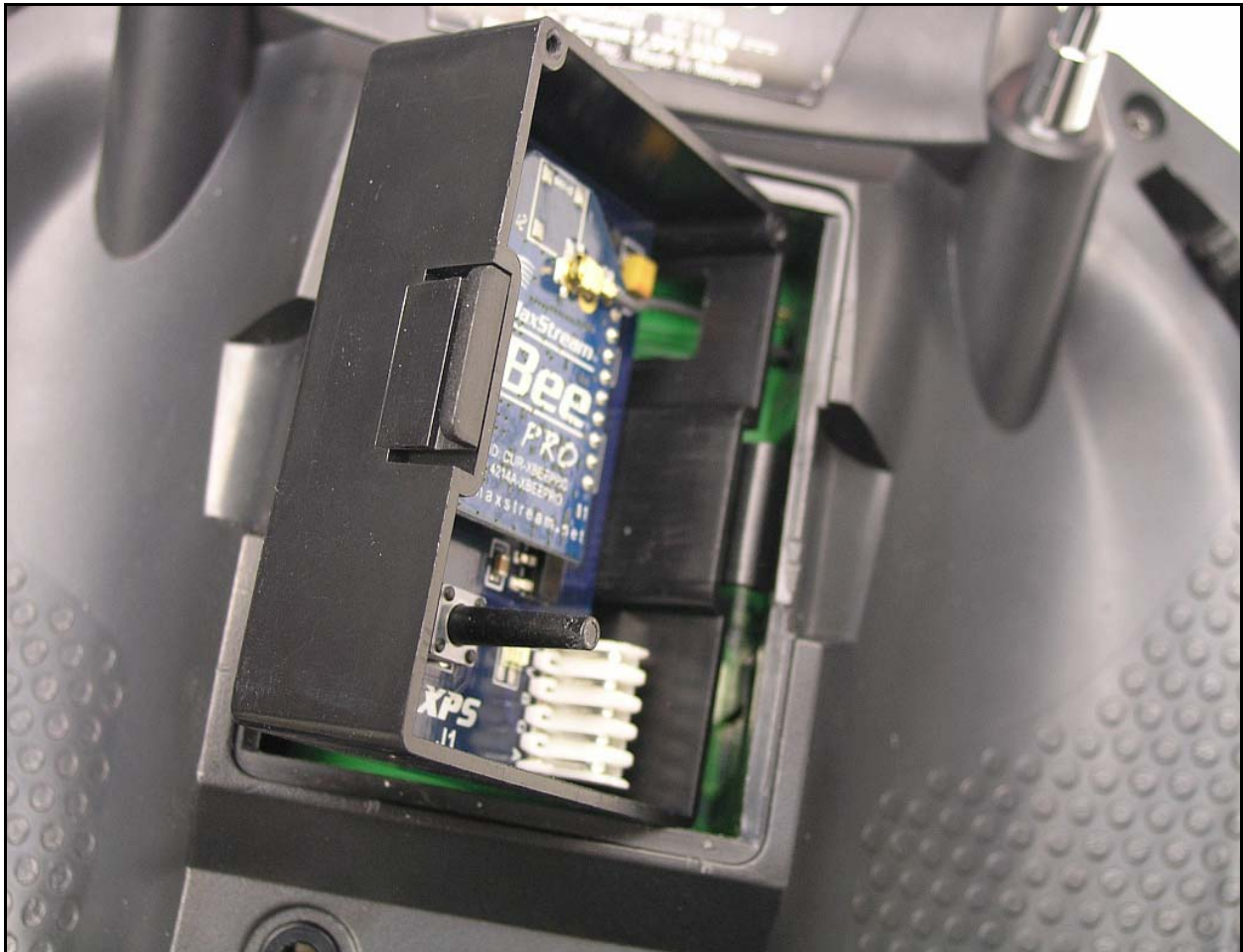
Figure 8 – Put the XtremeLink® RF module fully into plastic case
