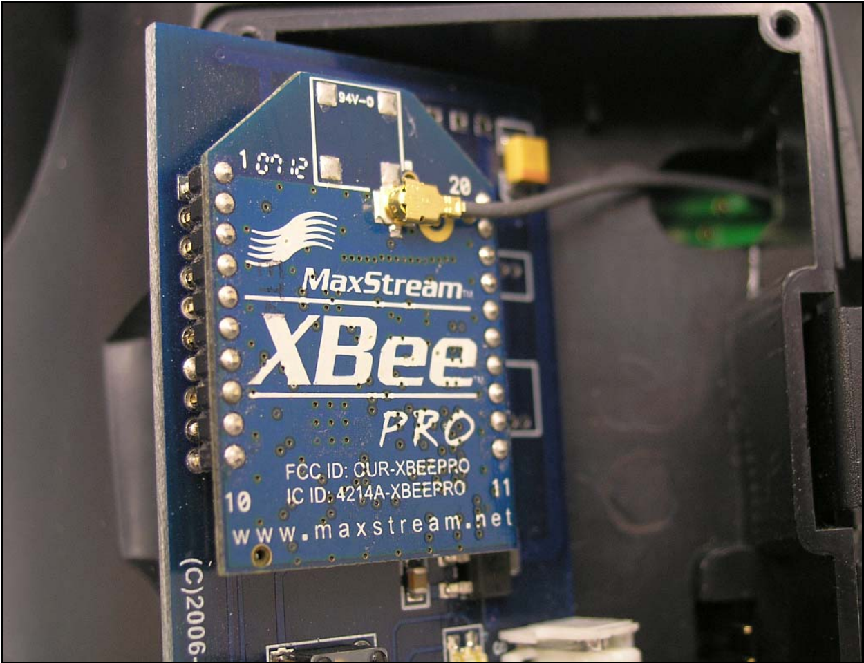
Figure 7 – Attaching antenna cable to XtremeLink® RF module
